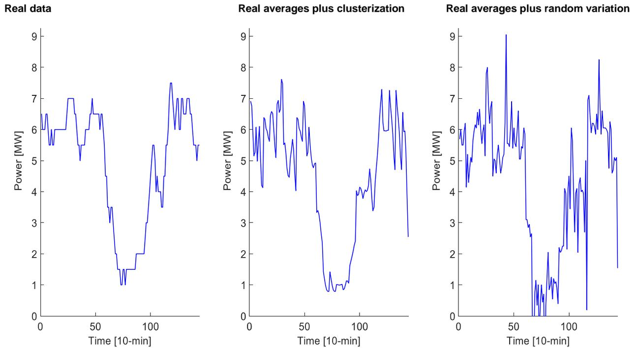
Figure 3-2: Wind profiles used in the autocorrelation test
