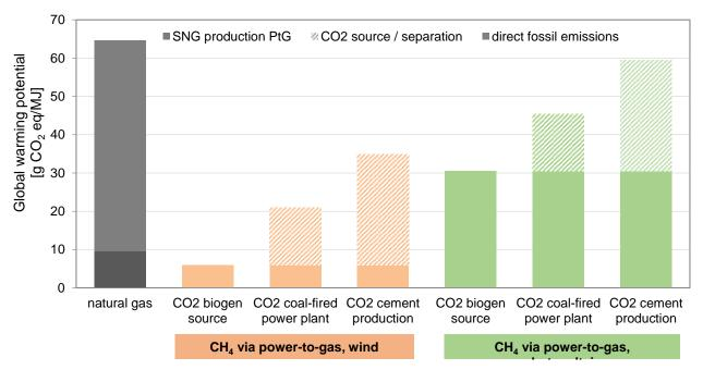
**Figure 4-3:** Global warming potential of CH<sub>4</sub> produced via power-to-gas with different electricity inputs compared to the benchmark technology steam reforming.
