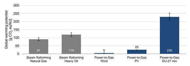
**Figure 4-6:** Global warming potential of H<sub>2</sub> produced via power-to-gas with different electricity inputs compared to the benchmark technology steam reforming (data from [69]).
