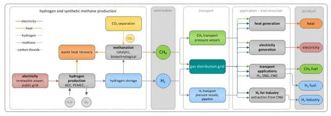
Figure 4-2: PtG system and system boundaries<sup>7</sup>
