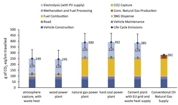
Figure 4-5: Greenhouse gas emissions of power-to-methane for mobility applications (produced by [65])
