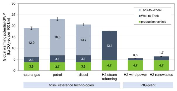
Figure 4-8: Results of the "well-to-wheel" analysis for hydrogen derived from PtG systems
