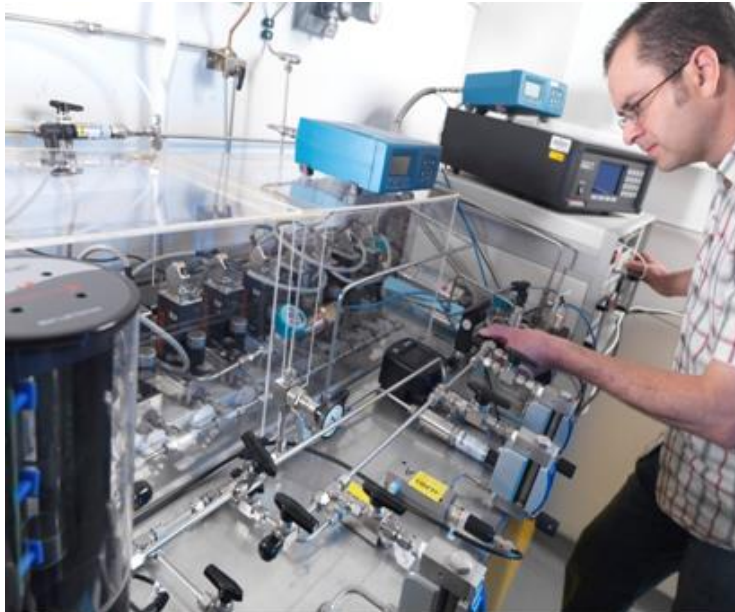
NPL multi-gas multi-pressure humidity generator
