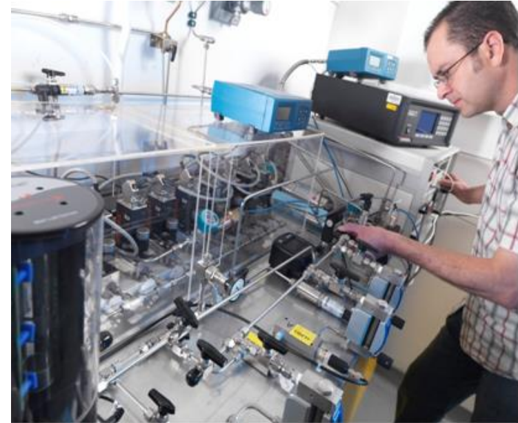
NPL multi-gas multi-pressure humidity generator
