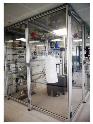
Figure 4: SSRT tensile, fracture and fatigue machine for testing in H<sub>2</sub> gas
