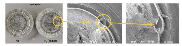
Figure 11: Fracture surface of notched SSRT x70 specimens tested in air and in H<sub>2</sub> (80 bar)
