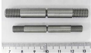
Figure 5: Notched round specimens for SSRT. Base (up) and welded (down) specimens from X70 steel grade
