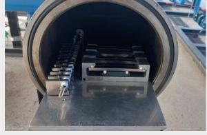
Figure 3: Insertion of strained specimens in the pig trap
