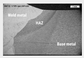
Figure 8: 4pb specimens after the 100% hydrogen campaign (left); detail of embedded cross sections (center); optical micrograph of X70 welded 4pb cross sections after the 100% hydrogen campaign (right)
