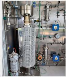
Figure 6: Gas separation prototype developed during HIGGS
