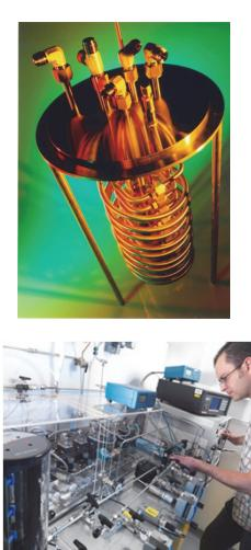
Figure 1: NPL facility for testing hygrometer response time to step changes in hydrogen water content
